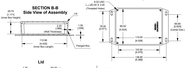
Purchased assembly includes box, lid and 4 cover screws. Box and lid are made from Diecast Aluminum Alloy. Silicone Gasket supplied with liquid resistant enclosure. Bottom Flange is Welded. **PART NUMBERS** 1590BBF Enclosure Natural Finish Enclosure Black Textured Enclosure 1590BBF Liquid Resistant Enclosure (Silicone Gasket) Natural Finish Enclosure 1590WBBFBK **Black Textured Enclosure**
