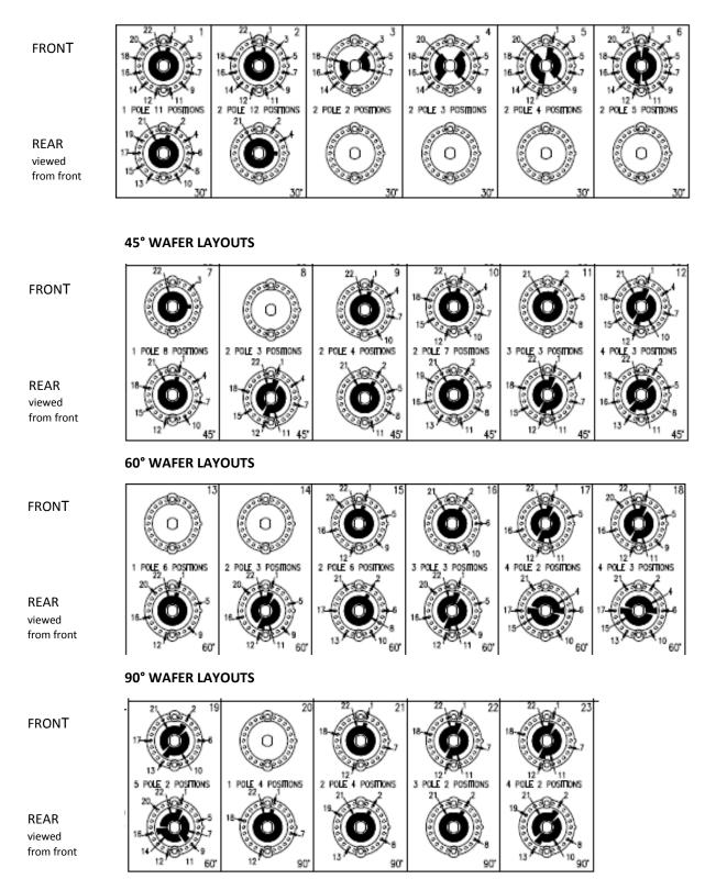
FRONT AND REAR WAFERS VIEWED FROM FRONT OF SWITCH IN FURTHEST COUNTER CLOCKWISE POSITION
