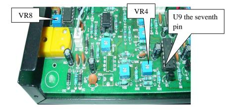
6. Switch PPM-200 "C-F" to "F" position. Repeat the steps from "1" to "3". Room temperature (F) 32(F)" should be displayed on the LCD screen.
