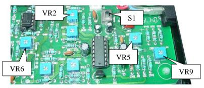
9. Dial S1 up, and input a signal (f 55hz, voltage value 10mV, 20mV, 30mV, 40mV, 50mV, 60mV, 70mV, 80mV, 90mV) ,the display will show the corresponding data. If it is not correct, please repeat step 1, 2, and 3 to check the calibration process.
