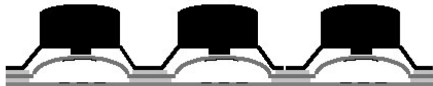
Membrane switch with silicone rubber keycaps
