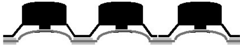
Keypads with poly-dome for tactile feedback
