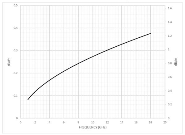
$^{1}$ Not including connector losses. Connector losses can be approximated as  $0.045x\sqrt{F(GHz)}$  dB/connector.
