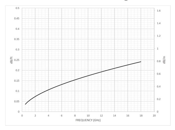
$^{1}$ Not including connector losses. Connector losses can be approximated as 0.045x√F(GHz) dB/connector.
