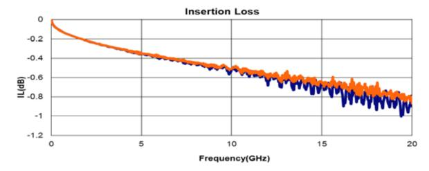
Typical. Results may vary. Includes cable assembly RF402-01RP1-01RP1-0305 (SMA to SMA, Right Angle) and adaptor effects. See characterization report for more information.
