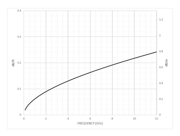
$^1\text{Not\,including\,connector\,losses}.$  Connector losses can be approximated as 0.045x $\sqrt{F(\text{GHz})}$  dB/connector.
