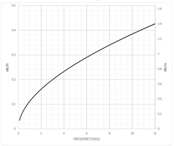
$^{1}$ Not including connector losses. Connector losses can be approximated as 0.045x√F(GHz) dB/connector.
