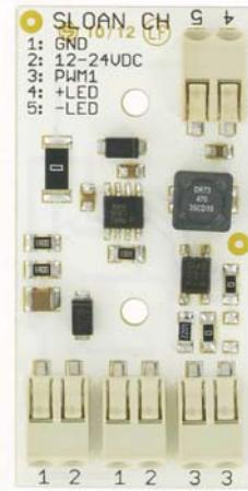
Input voltage must be 3V higher than the sum of the connected LEDs
