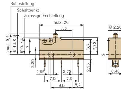
Abmessungen in mm
