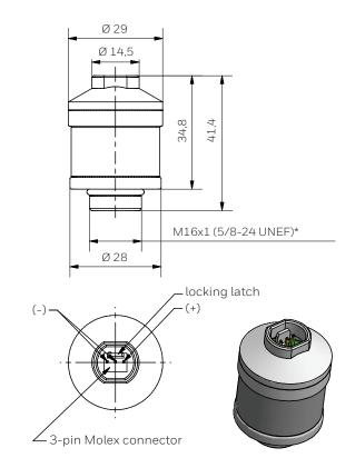
General tolerances ISO 2768-c \*Intermediate thread: Metric/Unified Extra Fine
